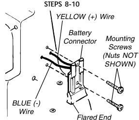
FIGURE 7 - INSTALLING THE BATTERY
